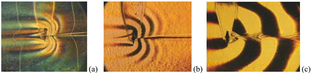
Fig. 5. Pattern of flow around a vertical strip ( H_c = 2.5 cm) moving from right to left; (a, b) – T_b = 12.5 s, U = 0.1 cm/c, “slit-thread” and “slit-knife” methods; (c) – T_b = 17.4 s, U = 0.3 cm/s, “slit-knife” method.
